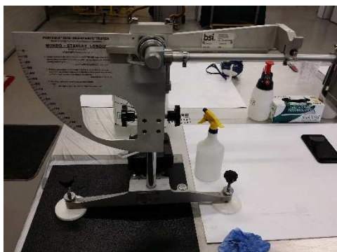
Image 1. Pendulum tester in-situ
