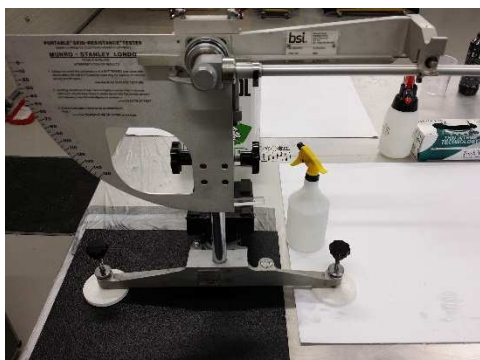
Image 1. Pendulum tester in-situ
