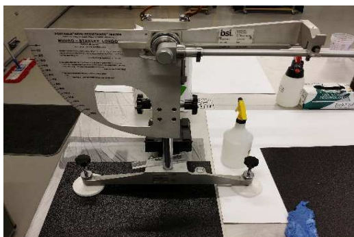
Image 1. Pendulum tester in-situ
